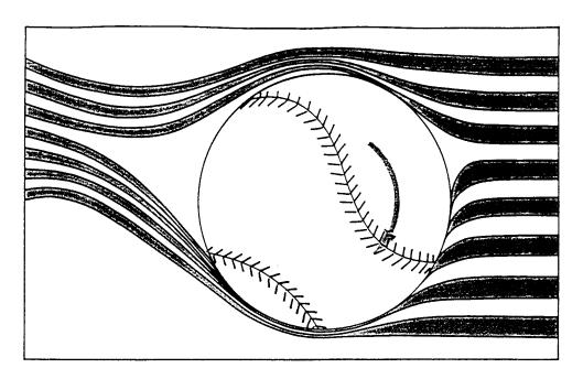
Spinning clockwise in a wind tunnel, a baseball disrupts the flow of smoke streams injected from the right. The stitches on the ball pull a thin layer of air around with them as they spin. This spinning layer causes more air to flow around the bottom than the top. The bottom air travels faster and thus makes the air pressure on the bottom of the ball lower, pushing the ball down. (Top-© Flash Fleischer. Bottom-© Prof. F. N. M. Brown of University of Notre Dame)
